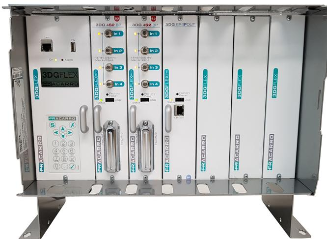
Example: 3DGFlex Evo headend composed by 2pcs of **3DG-4S2-BP** quad DVB-S2 receivers and 1pc of **3DGBP-IPOUT** IPTV streamer
