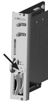
To remove the CAM, press the corresponding button
