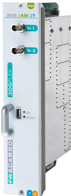
Fracarro's twin ASI - DVBT/C module, part of the 3DGFLEX range, allows you to simultaneously receive programs from up to 3 different sources (two independent ASI sources connected through the BNC front connectors and one transport stream available through the back panel).
